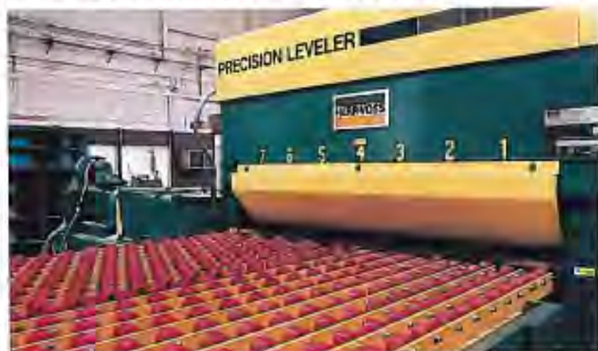
▲ Staggered skate wheels on inspection table downstream of Herr-Voss leveler prevent strip sagging; hold metal flatter than full-width rolls. Wheel material is non-marking polyurethane.
