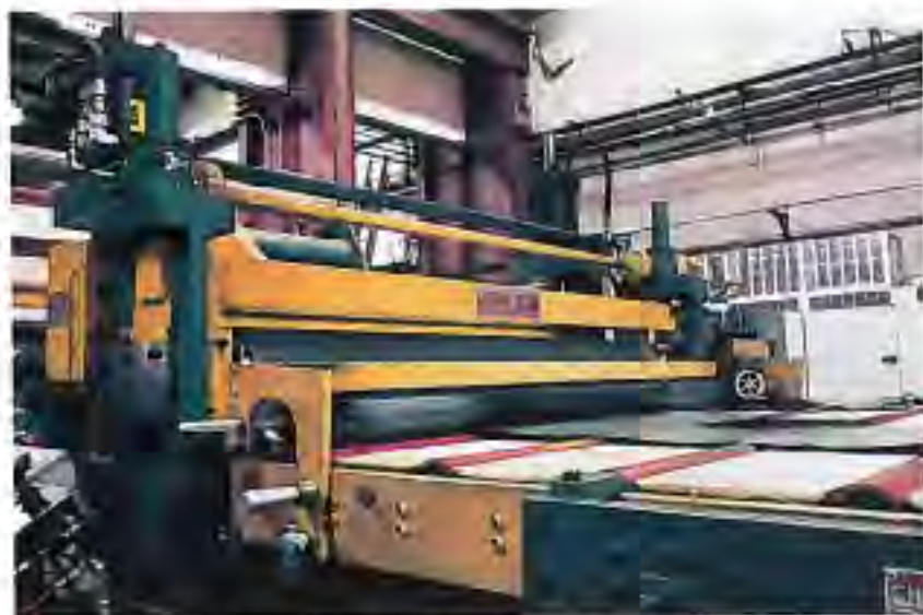
▲ Tension stand uses nonwoven fabric rolls to prevent scratching steel that will be coated with porcelain enamel for home appliances and related products.
